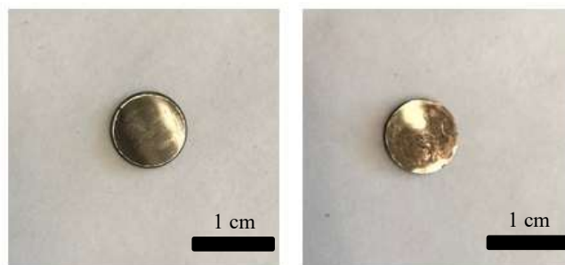
Figure 24. Comparison of an unaltered mica disk (left) and a mica disk with an added hydrophobic barrier (right)
